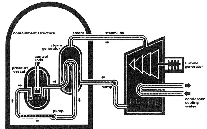
Pressurized water reactor (PWR). The water in the pressure vessel circuit is kept under pressure so that it does not turn into steam at high temperatures. In a boiling water reactor (BWR) there is no heat exchanger (marked “steam generator” above); the steam from the pressure vessel goes directly into the turbine, and the water from the condenser goes directly back into the pressure vessel.
